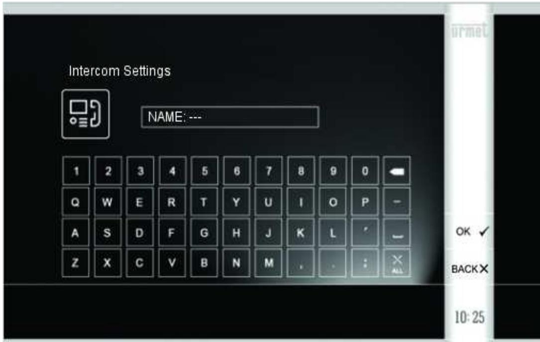
In this page, a name can be associated to the selected monitor via the keypad.
